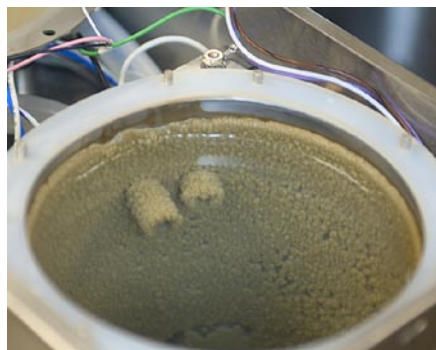
Water tank without Scale-Pro in use.*
